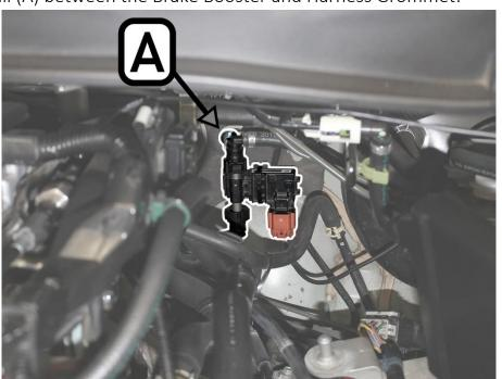
• To do this, simply place the slotted bracket onto the stud and use the provided M6 Nut to secure the bracket in place.
