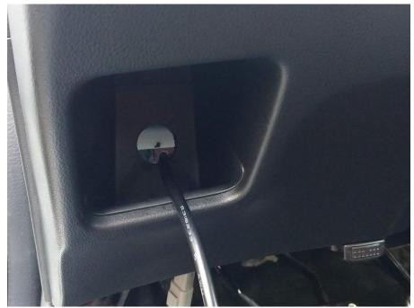
5. Continue by routing the ECT2 Male Connector from the Flex Fuel Chassis Harness to the engine bay. A good option is to pass it through the door jamb grommet, found to the bottom of the hood latch release cable grommet.
