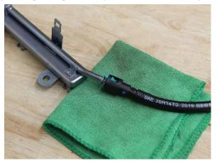
6. Hold the connector (A) with one hand and squeeze the retainer tabs (B) with the other hand to release them from the locking tabs (C).
